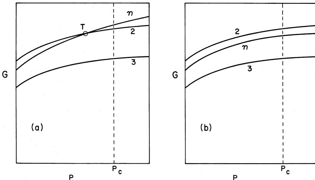
FIG. 8.—Schematic plots of the Gibbs potential per baryon vs. pressure ( $P$ ) for neutron matter ( $n$ ), two-flavor quark matter (2) and strange matter (3). The dashed line at  $P = P_c$  corresponds to the central density of the star. In case (a) a first-order phase transition occurs at  $T$ ; there is no such transition in case (b).
