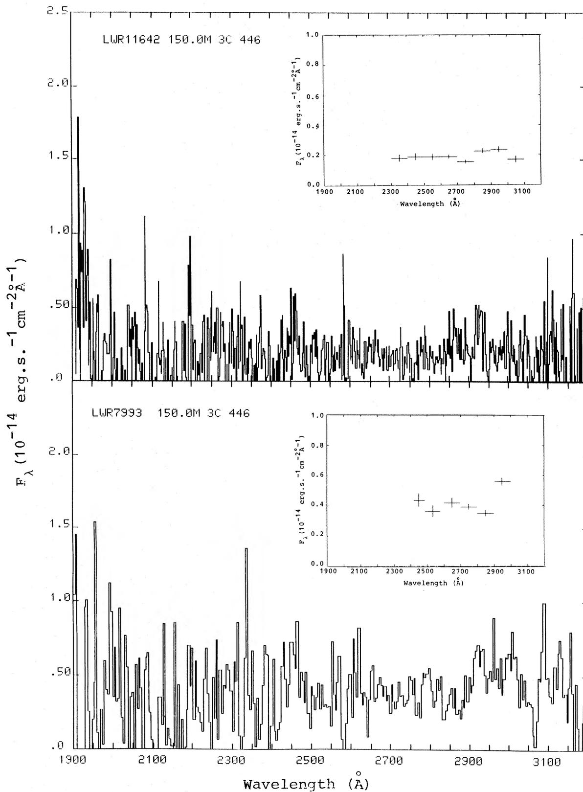
FIG. 3.—Ultraviolet spectrum of 3C 446. (top) 1981 September, (bottom) 1980 June. The inserts show the 100  $\text{\AA}$  binnings used to fit the data.
