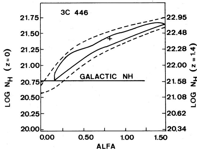
FIG. 2.—90% (solid line) and 99% (dashed line) two-parameter confidence contours for the X-ray spectrum shown in Fig. 1. The plus indicates the best-fit value, and the horizontal line the amount of Galactic hydrogen as computed from Burstein and Heiles (1982). The left-hand scale gives the  $N_H$  corresponding to a cutoff energy at  $z = 0$ , while the right-hand scale gives the  $N_H$  corresponding to a cutoff energy redshifted to  $z = 1.414$ .
