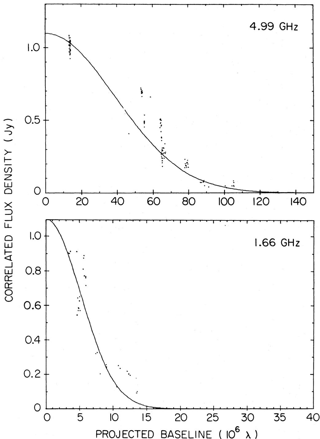
FIG. 2.—Observations of 2013+370 at 4991 and 1663 MHz. Plotted are the correlated flux density vs. projected baseline length (in millions of wavelengths). Solid curves represent Gaussian models with diameters (FWHM) of 2 and 15 mas.
