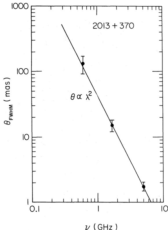
FIG. 3.—Measured angular size of 2013+370 as a function of frequency. The data show the angular size scaling as the square of the wavelength, as expected for scattering.
