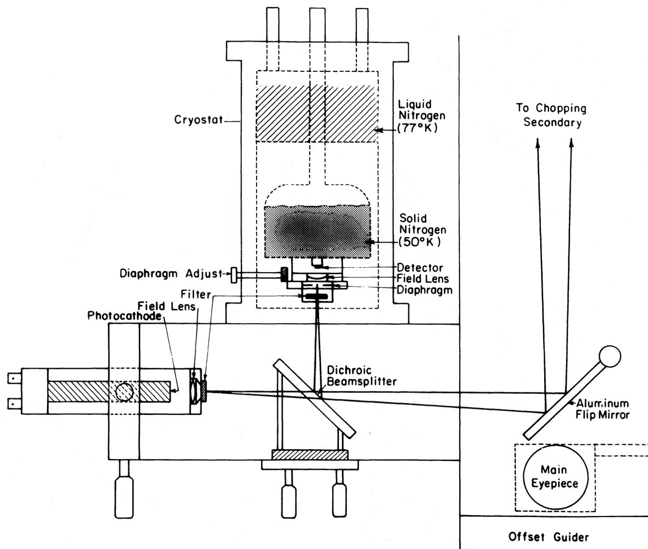
FIG. 1.—Schematic diagram of infrared/optical detection system. Diagram shows visual phototube and cryostat with an infrared detector. Dichroic beam splitter provides simultaneous measurements in visual ( $V = 5500 \text{ \AA}$ ) and  $2.2 \mu\text{m}$  ( $K$ ) photometric bands through diaphragms aligned in focal plane of telescope.
