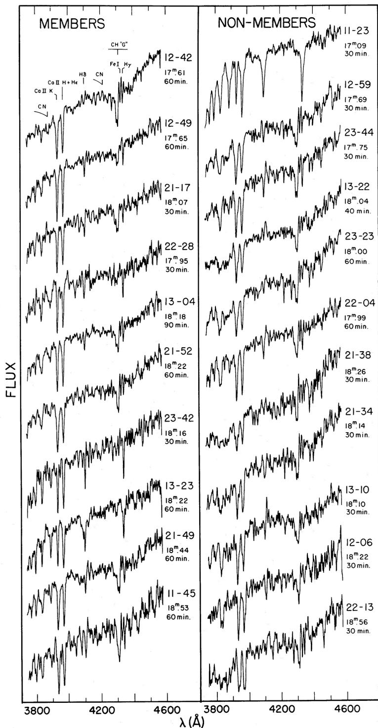
FIG. 5.—A spectral montage of flux (linear but arbitrary scaling) vs. wavelength for stars observed in 1981. With the exception of the upper two member stars, all spectra were obtained under photometric conditions. The observed  $B$  magnitude and the exposure time in minutes are given below each star name. Spectra of additional faint member stars observed in 1980 are given in Paper I.
