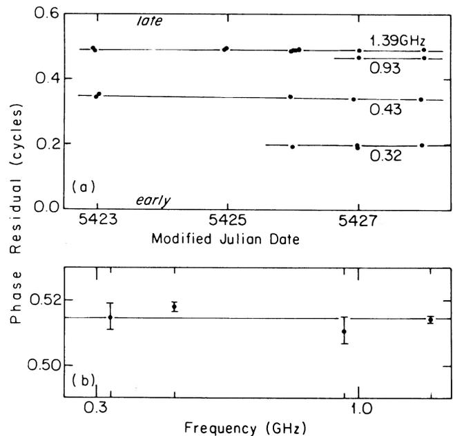
FIG. 4.—(a) Residual phase vs. Julian date for four radio frequencies using nominal parameters. (b) Residual phase vs. frequency after correcting phases in (a) for errors in rotation frequency and dispersion measure.
