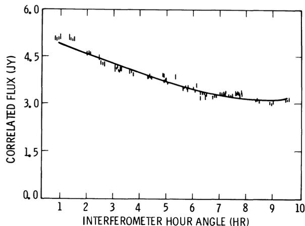
FIG. 2.—Correlated flux density on Parkes/Tidbinbilla baseline as a function of interferometer hour angle. Solid line indicates the best fit elliptical Gaussian model.
