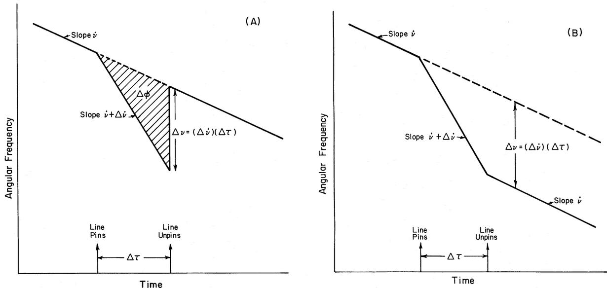
FIG. 5.—Illustrating the characteristic signature of a pinning event. If, upon unpinning, the line returns to the position it would have had if it never pinned at all, (a) applies; (b) applies if it does not.
