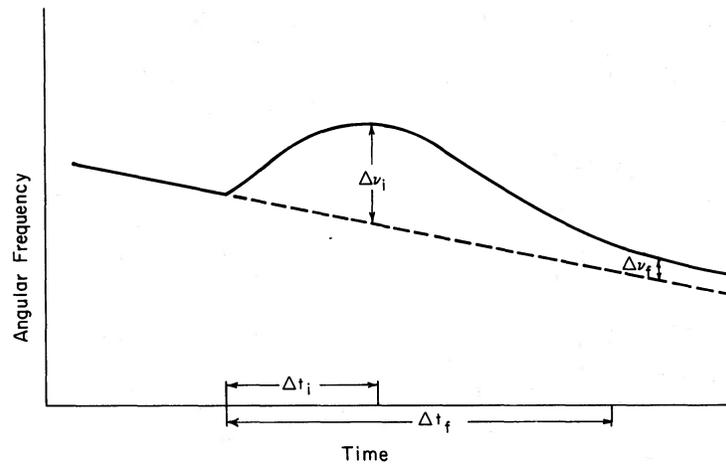
FIG. 6.—Illustrating the characteristic signature of a spin-up.
