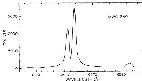
FIG. 2.—The echelle spectrum of MWC 349 showing  $H\alpha$  and  $[\text{N II}]$ . The central reversal of  $H\alpha$  is blueshifted by  $\sim 15 \text{ km s}^{-1}$  from its center of symmetry.
