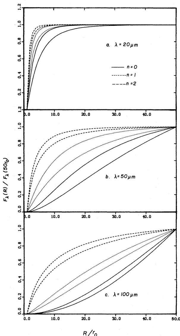
FIG. 4.—Relative flux density as a function of cloud size at 20, 50, and  $100\ \mu\text{m}$ . Each graph shows the effects of density gradient ( $n$ ) and temperature gradient ( $\beta$ ) on the flux dependence on  $R$ . The upper curve of each pair is for  $\beta = 0.38$  and the lower curve  $\beta = 0.33$ .  $T_0$  is chosen to be  $125\ \text{K}$ .
