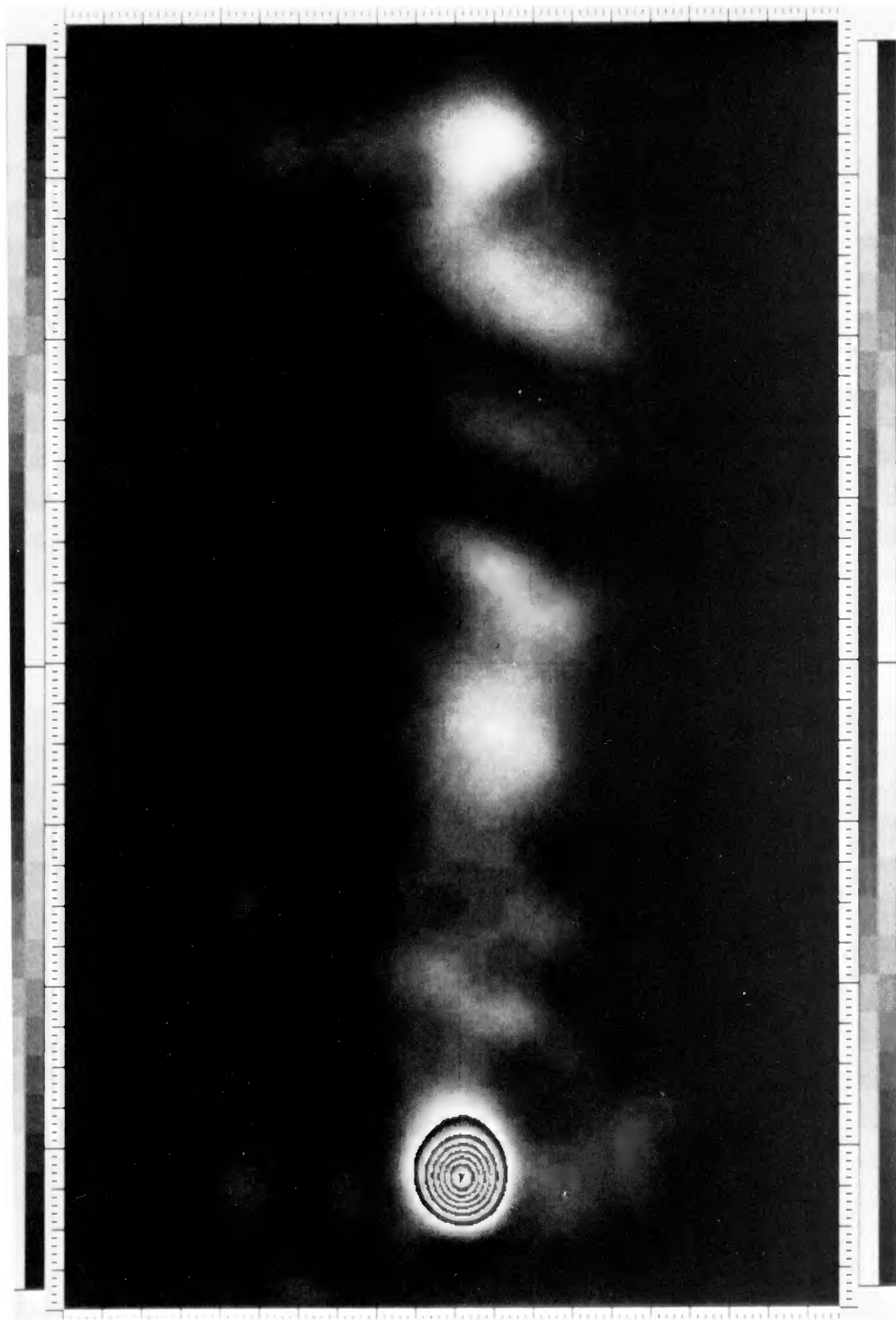
FIG. 2.—“Radio photograph” from hybrid map of Fig. 1 a . The source has been rotated counterclockwise by 35^\circ . The brightness temperature was scaled to produce numbers in the range 1 to 128, and the three most significant bits were then clipped. This gives the full range of the gray scale (16 levels) to the features in the jet, and produces the dark rings in the core. Thus the brightest features in the jet are about one eighth of the peak brightness of the core, and the successive dark rings are contours at one, two, . . . , etc., eighths of the peak core brightness.
