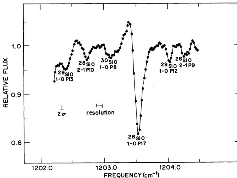
FIG. 1.—Observed spectrum of VY CMa near  $1203\text{ cm}^{-1}$  ( $8.31\text{ }\mu\text{m}$ ). The instrumental transmission has been removed. A weak telluric absorption line occurs near  $1202.4\text{ cm}^{-1}$ . Spectral resolution and random noise are as shown.
