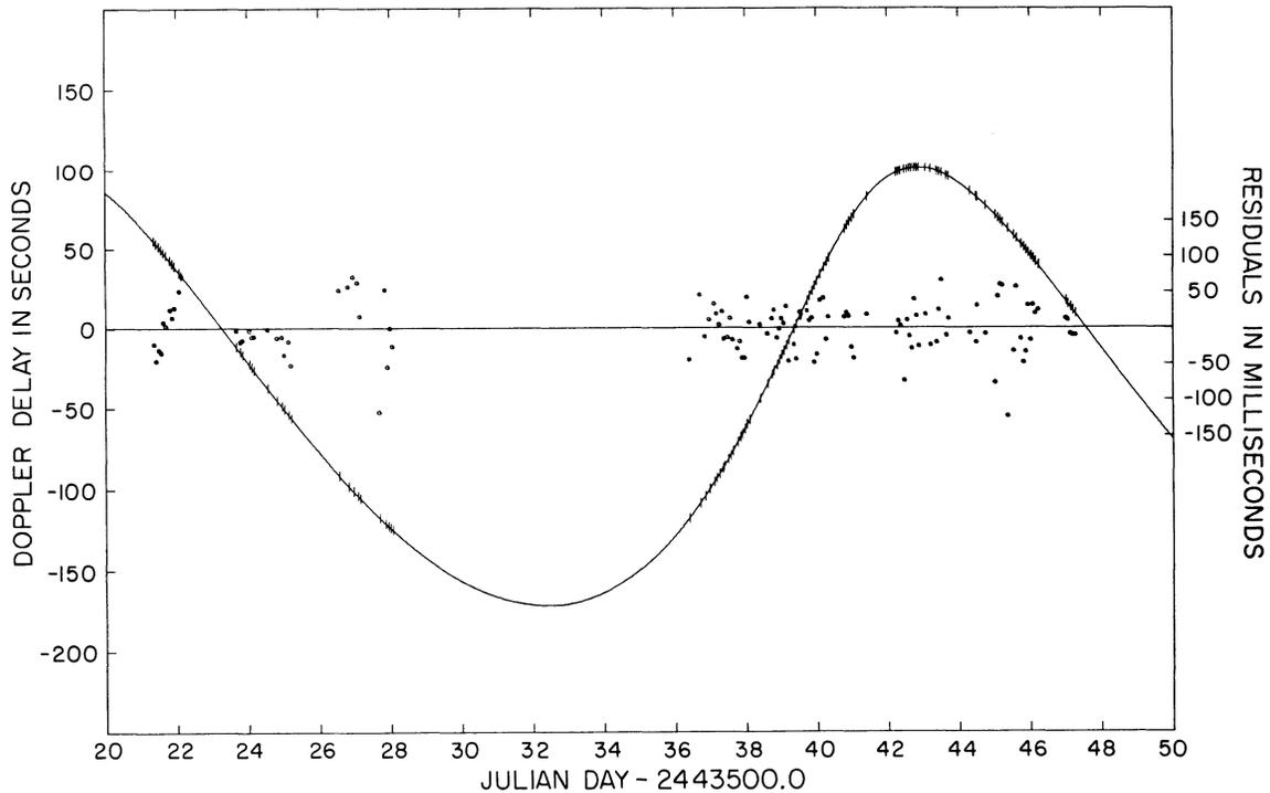
FIG. 1.—Doppler delay data for 4U 0115+63. The vertical bars are the measured delays in pulse arrival time (*left-hand scale*); the length of each bar is considerably larger than the uncertainty in the measurement. The solid curve represents the expected delays for the best-fit orbital parameters given in Table 2. Small open circles (*right-hand scale*) indicate the residual differences between the measured delays and the best-fit curve.
