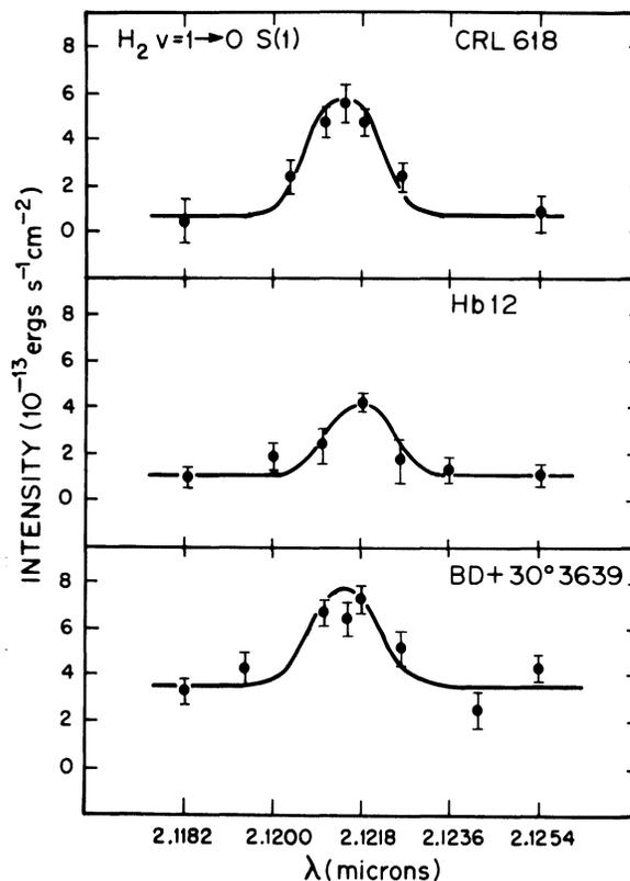
FIG. 3.—The measurements of BD+30°3639, Hb 12, and CRL 618 made with the grating spectrometer system. The intensity and wavelength scales are the same for all plots. The continuum flux level was determined by averaging the points that are  $18\ \text{\AA}$  or more from the line center. In each case the measured instrumental profile, appropriately normalized and centered, has been drawn through the data to aid the eye.
