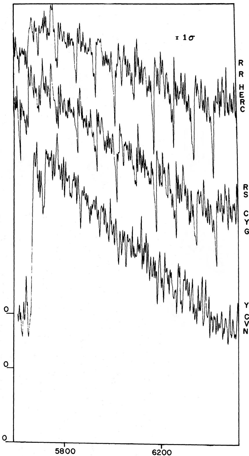
FIG. 1.—Spectra of RR Her, RS Cyg, and Y CVn from  $5600\text{ cm}^{-1}$  to  $6500\text{ cm}^{-1}$ . The spectra are normalized to the highest continuum point but have offset zeros indicated in the figure for clarity. The strong absorption at  $5656\text{ cm}^{-1}$  is the  $\text{C}_2$  Ballik-Ramsay band. The vertical scale is linear in relative flux per wavenumber.
