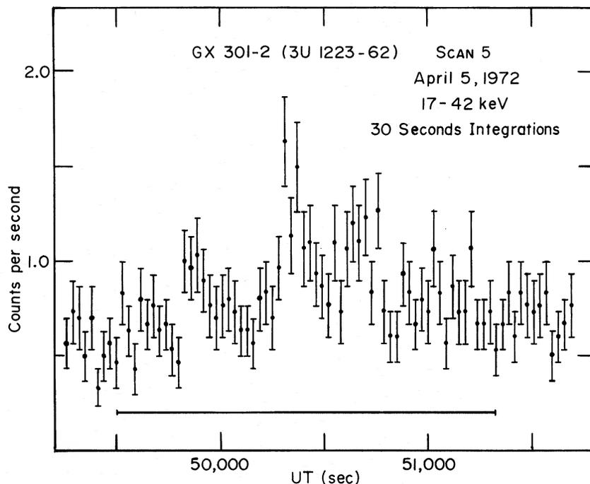
FIG. 5.—Counting rate versus time for scan 5. Each data point represents the counting rate observed in a 30 s period ( $\pm 1 \sigma$  error bars). The horizontal bar indicates the time during which 3U 1223-62 was in the field of view of our detector. The source flux is varying continuously. A large change of at least a factor of 5 is observed near UT 50,250 s.
