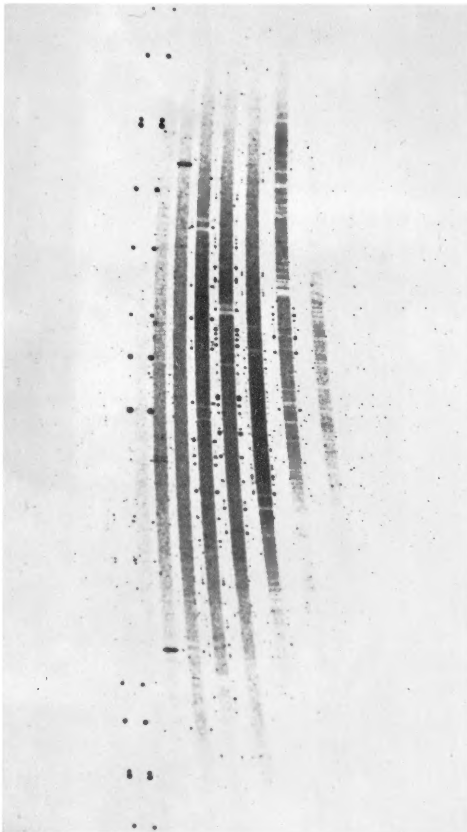
FIG. 2.—A reproduction of spectrogram SI 868 of 1331 + 170. The strong emission lines in the 9th and 11th orders are due to C IV \lambda 1549 and L\alpha , respectively, at z = 2.081 . The C IV absorption doublet at z = 1.7754 appears in the 10th order. The strong nightsky emission in the 7th and 8th orders is O I \lambda 5577, and the nightsky Na I D lines are seen clearly resolved in the 7th order.
