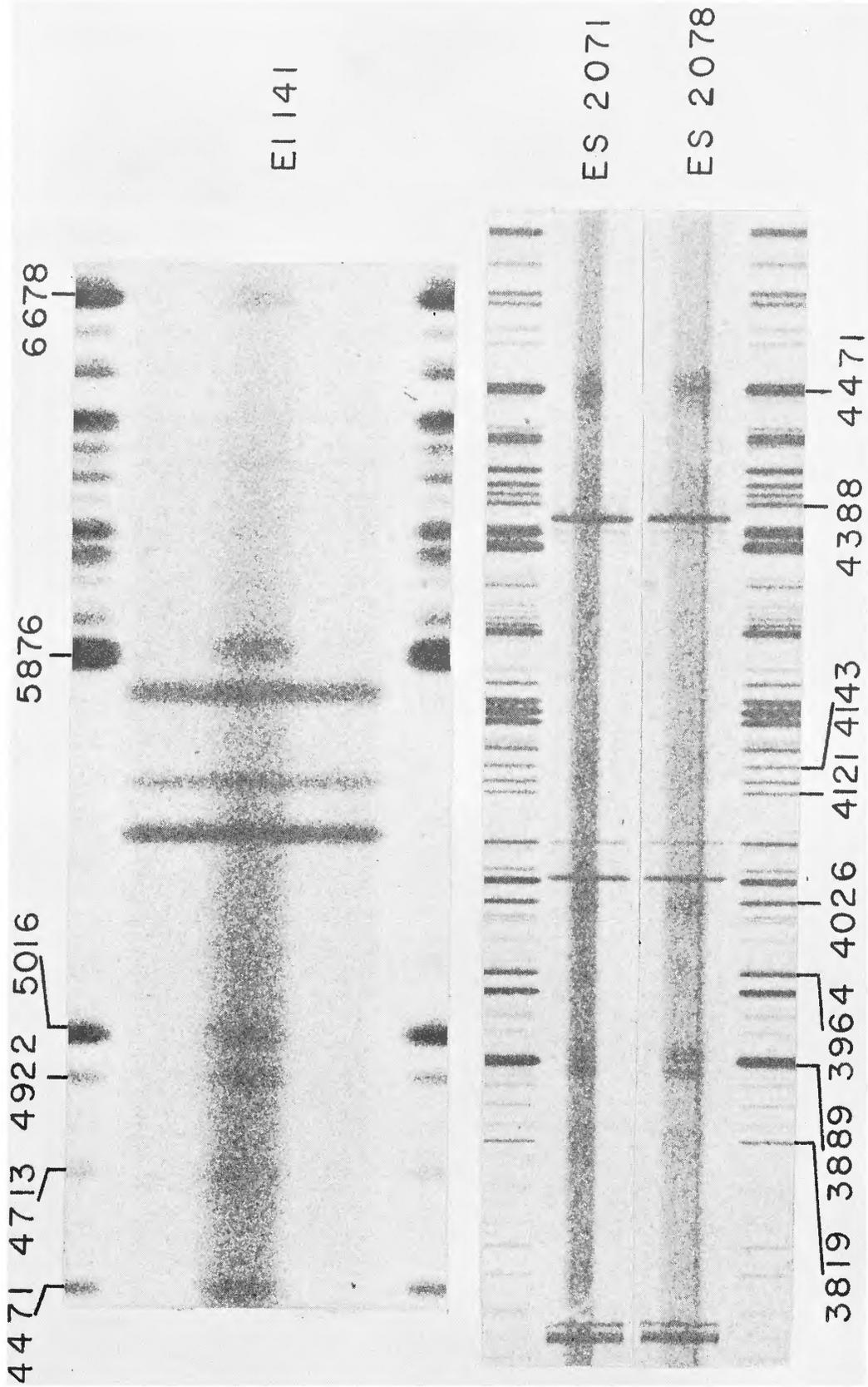
FIG. 1.—Spectrograms of G61-29 obtained at prime focus of the Lick 120-inch telescope, EI 141 with Carnegie image-tube spectrograph, ES 2071, 2078 with photographic spectrograph. Several He lines in the comparison spectra are marked where broad He emission lines can be seen in the star. Lines crossing the whole object window in each spectrogram are Hg lines from city lights and [O I]  $\lambda$ 5577. Note structure in He I  $\lambda$ 3889 and 4471 in the star in ES 2071 and 2078.
