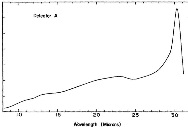
FIG. 5.—The sensitivity function of the spectrograph (detector A)
