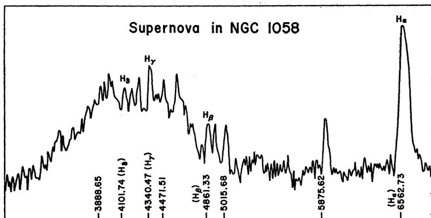
FIG. 2.—Direct tracing of a spectrogram of the supernova in NGC 1058 obtained with the 200-inch prime focus spectrograph on February 1, 1962. Emulsion 103a-F, dispersion 400 Å/mm, exposure time 65 min at seeing 3. In addition to the Balmer lines, which are indicated, many emission lines due to He I and Fe II are clearly discernible.
