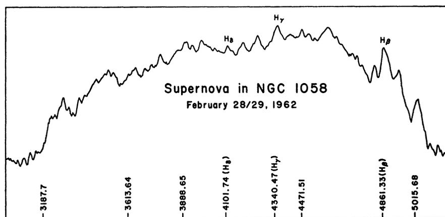
FIG. 3.—Direct tracing of spectrogram of the supernova in NGC 1058 obtained with the prime-focus spectrograph of the 200-inch telescope on February 28, 1962. Emulsion IIa-O, dispersion 400 Å/mm, exposure time 90 min at seeing 3. The same features are discernible as in the blue region of the tracing reproduced in Figure 2
