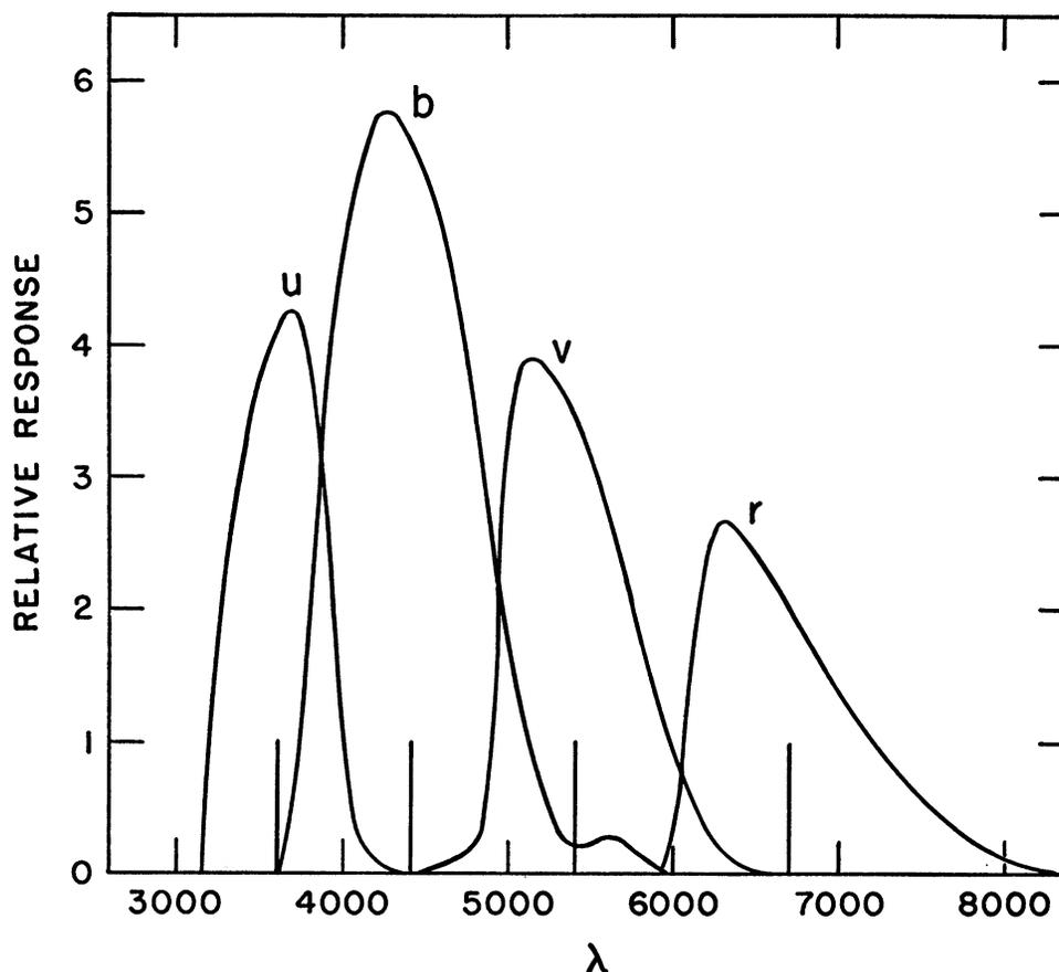
FIG. 1.—The transmission function  $S(\lambda)$  for the filters, S20 photocathode, and two reflections from Al. The filters are 2.8 mm of Corning 9863 plus 2.5 mm of 80 per cent saturated  $\text{CuSO}_4 \cdot 5 \text{H}_2\text{O}$  solution for  $u$ ; 0.7 mm of Schott BG12 plus 2 mm of Schott GG13 plus 2.5 mm of 80 per cent saturated  $\text{CuSO}_4 \cdot 5 \text{H}_2\text{O}$  solution for  $b$ ; 1.6 mm of Schott BG18 plus 2.2 mm of Schott GG11 for  $v$ ; and 2 mm of Schott RG1 for  $r$ .
