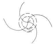
FIG 6—Projection onto the solar equatorial plane of the lines of force of any solar field which is carried to infinity by outward-streaming gas with velocity  $10^3$  km/sec
