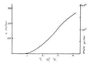
FIG 5—Steady outward velocity at  $a = 10^{11}$  cm and the resulting solar mass loss if the hydrogen density is  $3 \times 10^7$ /cm<sup>3</sup>, as a function of coronal temperature
