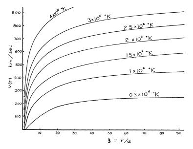
FIG. 1 —Spherically symmetric hydrodynamic expansion velocity v(r) of an isothermal solar corona with temperature  $T_0$  plotted as a function of r/a, where a is the radius of the corona and has been taken to be  $10^{11}$  cm
