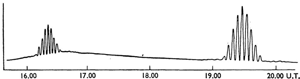
FIG. 3.—Section of record obtained with spaced-aerial interferometer, showing the intense radio stars in the constellations of Cygnus (16.20) and Cassiopeia (19.30).
