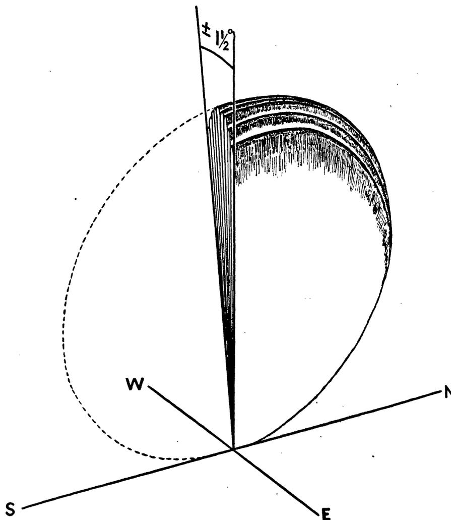
FIG. 2.—*Reception pattern of spaced-aerial interferometer.*
