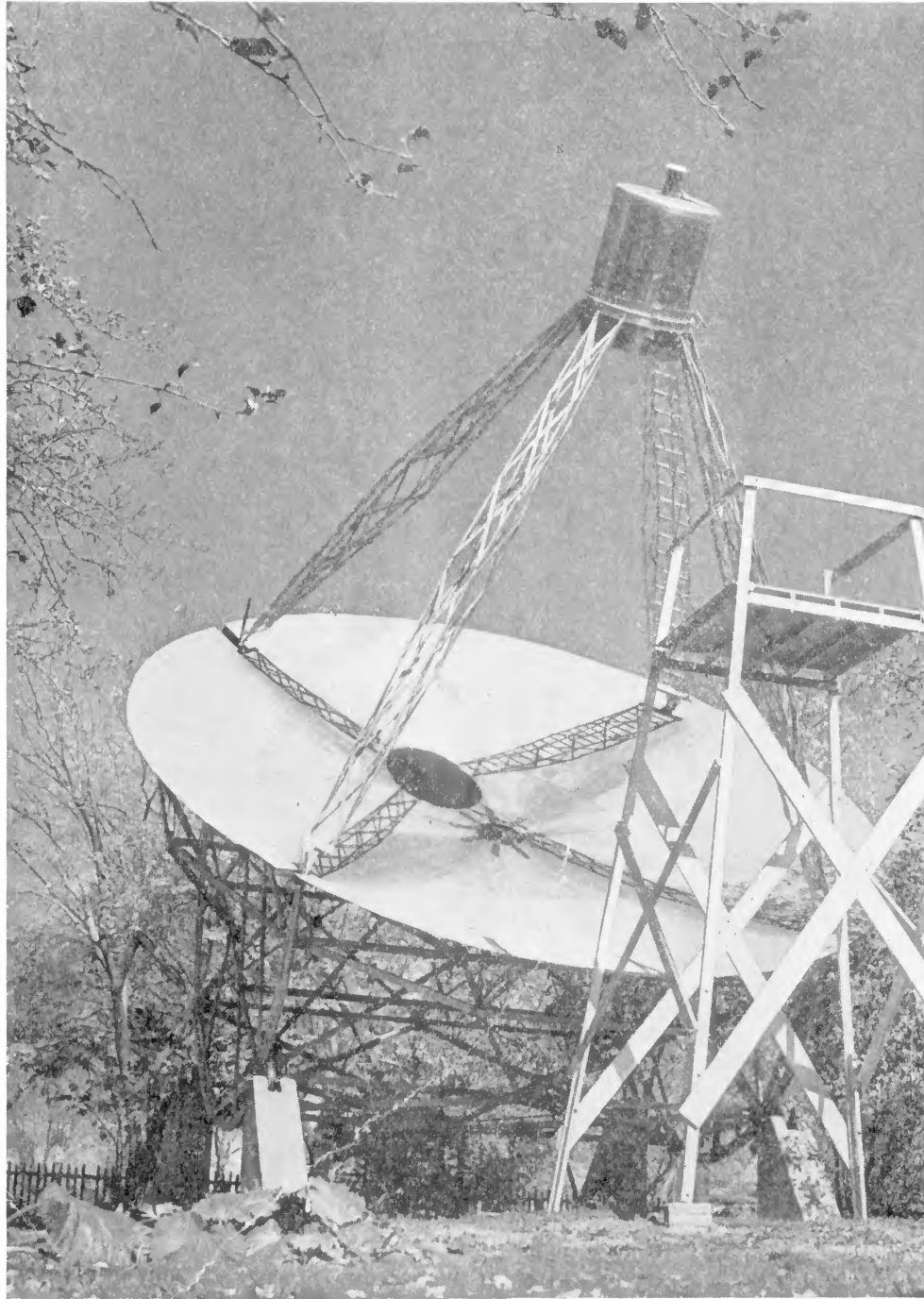
FIG. 1.—Sheet-metal mirror, 31.4 feet in diameter, 20 feet in focal length, used for collecting cosmic static
