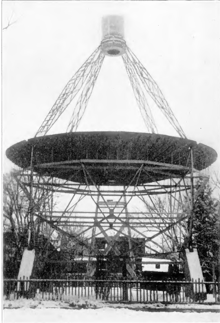
FIG. 1.—Antenna system viewed from the north. The resonance chamber can be seen supported at the focal point of the parabolic reflector.
